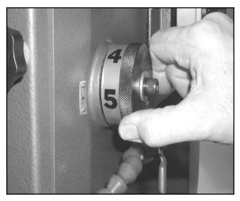
Figure 19. Depth control ring.
